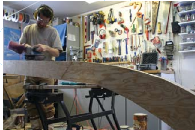
On the curve: Hugh Dale-Harris shown in his workshop shaping the runner for the sleds. The runners were fashioned after Peary's design. The crew strapped two runners together to ensure a parallel shape
